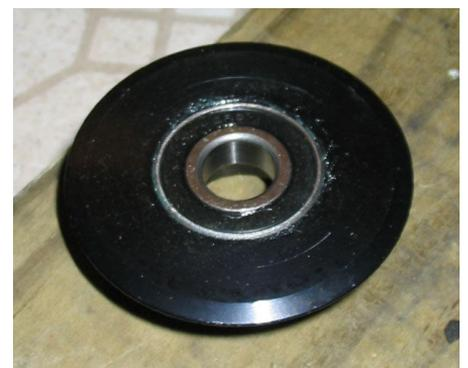
Remember that axle you hammered out earlier? Well grease it up and push it into the inner race of the bearing you just hammered in!
