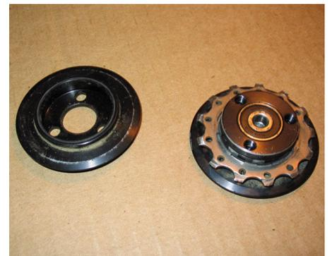
Now that you have the machined pulley sides apart, take a look at the piece that holds the bearings. There will be two bearings, one large with a metal axle insert and one small bearing. These two bearings are separated by a metal wall so you cannot simply hammer the smaller one directly against the larger bearing and make it pop out.
