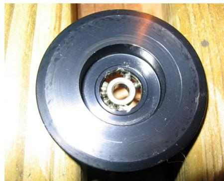
To remove the smaller bearing, find something about the size of the internal race. In my case I use a socket wrench extender.
