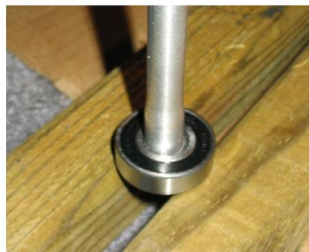
Notice the axle has a lip on it on one side. Make sure you are not trying to hammer it out the wrong.
