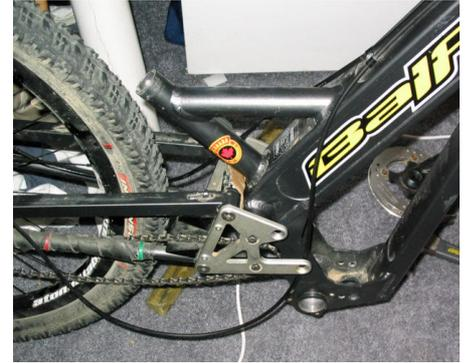
The first step to disassembling all this is to remove the rear triangle and the two screws that hold the pivot together. If you find you cannot unscrew both linkage plates, don't worry about it, only one needs to be unscrewed now.
