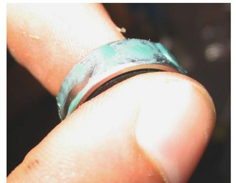
With the bearing greased up, use a hammer and dowel or a vice to squeeze it back into the cup it sits in. As with the larger bearing, make sure you don't harm the rubber seal!
