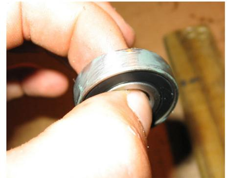
You will need to hammer (or push back into place with a vice) the big bearing back into the cup it sits in. Make sure that you do not damage the rubber seal of the bearing while doing this. If you have to hammer it back in, try using a dowel or piece of wood that covers the surface of the bearing. This will help distribute the force in addition to preventing you from mashing in the rubber seal.
