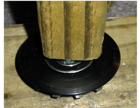
Find the smaller bearing and lubricate it. As with the larger bearing, the grease will help cut down on squeaks and also aid in future removal processes.
