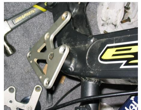
With the axle in, all you need to do for the other side (the side with the pulley) is to grease the divet in the linkage plate the axle is pushed into, add the washer, then screw the pivot bolt back in.
