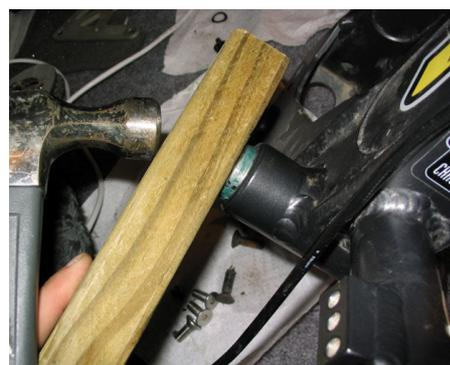
It took me a while to tap the bearing in... Make sure that it is flush with the frame then wipe off the excess grease. After you are done with this, repeat this process for the other side.
