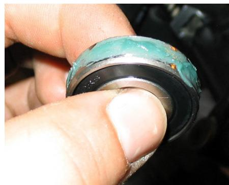
With the bearing greased up, insert it into the cup and then using a hammer and dowel, tap it in. Make sure that you do not damage the rubber seal of the bearing while you do this.
