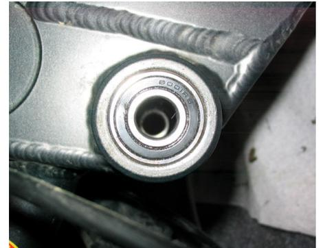
You can see in this picture that I hammered the axle through without a screw. I was able to avoid mashing the threads by putting a socket atop of the cone in a manner that did not mash the threads. But if I were to do it again, I would have threaded a screw in.
