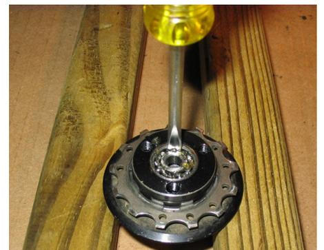
Below is a picture of the results of the hammering. As you can see, the screwdriver is still stuck in the races of the smaller bearing.
